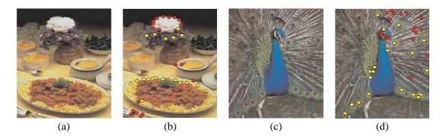
Fig. 3. (a) and (c) Corel images. (b) and (d) results of Harris detector (red dots) and the Harris detector with color boosting (yellow dots). The red dots mainly coincide with black and white events, while the yellow dots are focussed on colorful points.
