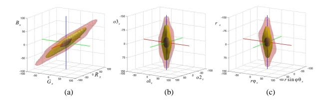
Fig. 1. The histograms of the distribution of the transformed derivatives of the Corel image database in respectively the (a) RGB coordinates, (b) the opponent coordinates and (c) the spherical coordinates. The three planes correspond with the isosalient surfaces which contain (from dark to light) respectively 90%, 99%, 99.9%t of the total number of pixels.
