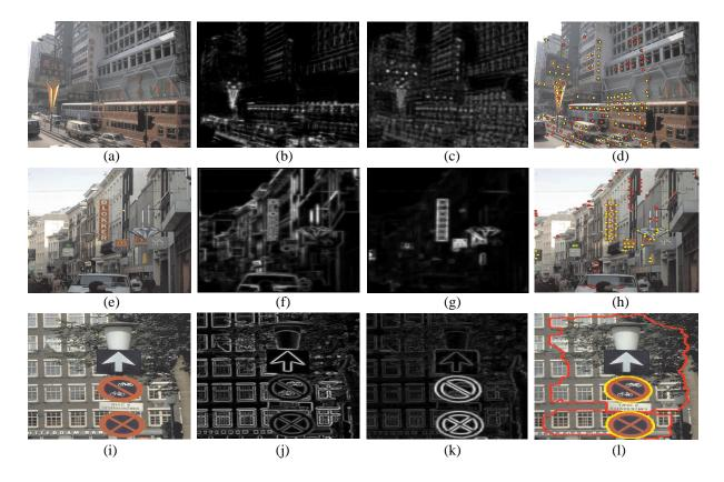
Fig. 6. Horizontally, respectively, the input image, RGB-gradient based saliency map, the color boosted saliency map and the results with red dots (lines) for the gradient-based method and yellow dots (lines) for the salient points after color saliency boosting. Row one (a,b,c,d): results after [11], row two (e,f,g,h): results after [16], and row 3 (i,j,k,l): results after [24]
