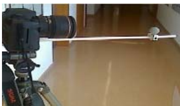
149 150 Figure 4: Camera and grey sphere setup.
