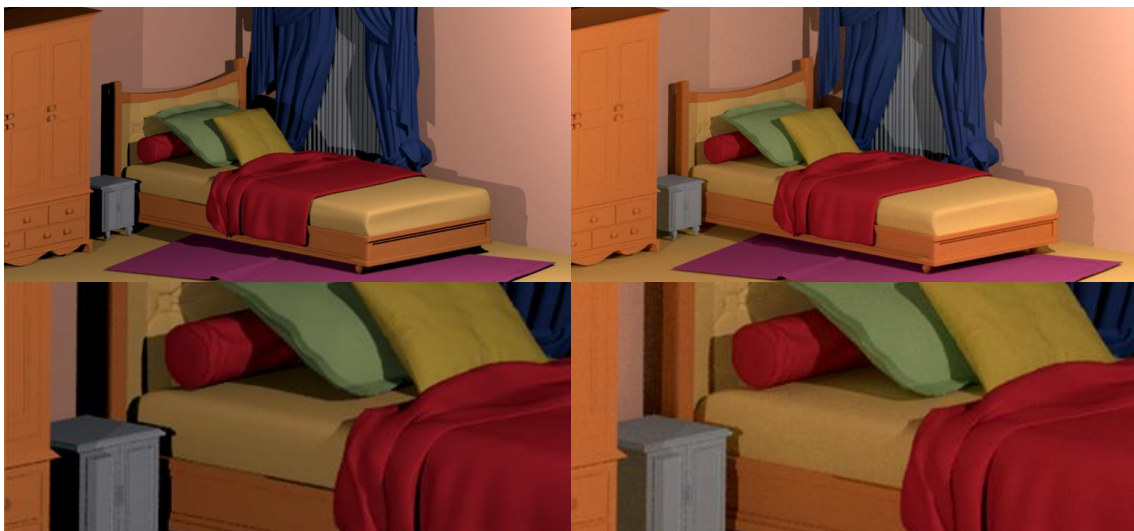
Figure 5.5: Comparing different rendering methods: direct lighting (left) and photon mapping (right) on an example scene from our dataset. Note that the gamma is added for visualization.
