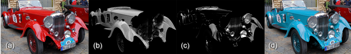
Figure 3.3: An example of intrinsic images recovered for an object. (a) Original image; Intrinsic images: (b) Body reflectance and (C) Specular reflectance; (d) An example recoloring result.
