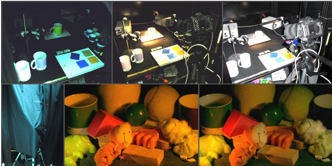
Figure 5.2: Here we demonstrate the process of data acquisition for our multi-illuminant scene images. The two images on the bottom right are examples of a complex scene (e.g., specular highlights and shadows) captured under distinct illuminants (note that these images are enhanced for visualization).
