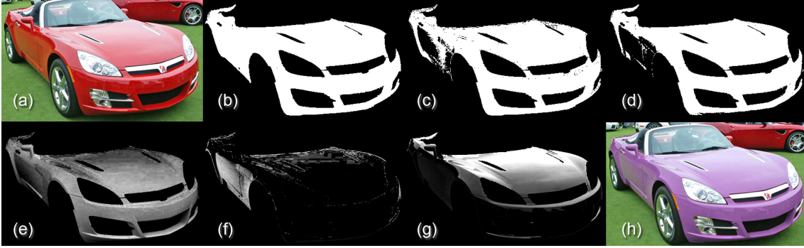
Figure 3.4: An example of the MIDR algorithm performance: (a) Original image; (b) Object mask as the initial Mask for the illuminant l_1 ; (c) The Mask after 1st iteration; (d) The Mask at 3rd (final) iteration; (e) estimated m_b^1 ; (f) estimated m_b^2 (the interreflection area, l_2 , has been correctly detected); (g) estimated m_s^1 ; (h) An example recoloring (the interreflection is preserved).
