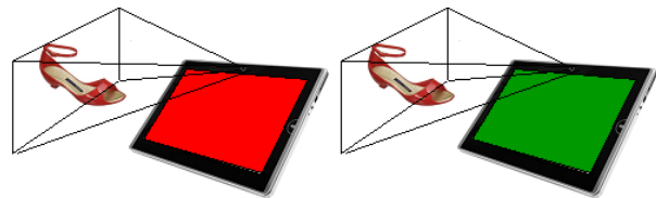
Fig. 1. Multispectral data can be obtained with hand-held devices by using the screen to illuminate the object under various illuminations. The acquired measurements can be used to reconstruct the spectral reflectance.
